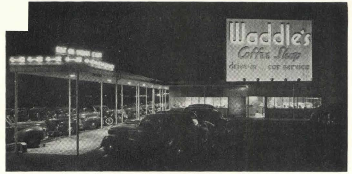
AT NIGHT, the big sign is floodlighted; downlights illumine the walk.
